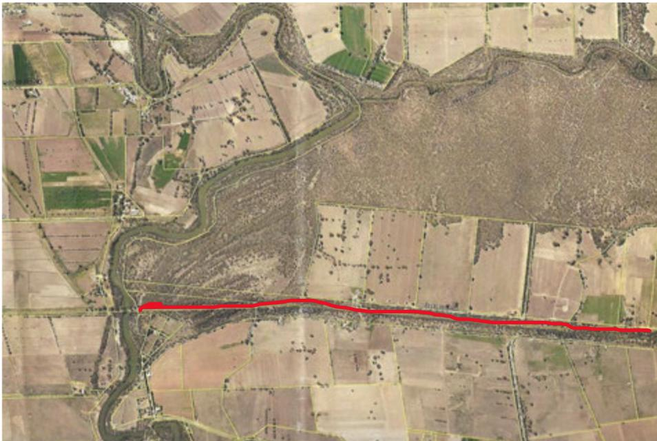
Above: Areal view, TIA Channel 2/4/1 > 3km (red line) showing vegetation on both sides of the channel. This channel was constructed to pump water using steam driven pumps from the Murray River into Gunbower Creek. The channel was dug out by men using teams of horse-drawn scoops in 1900c.
