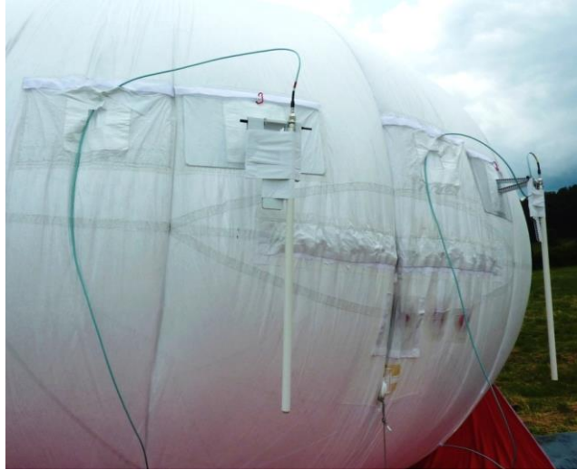
Stern View of ABSOLUTE Helikite showing 4G Radio equipment'
