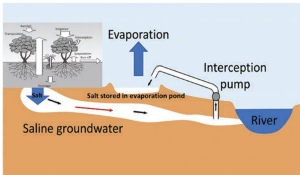
Figure 5. Schematic diagram of a salt interception scheme (redrawn from Williams, Walker, and Hatton 2002).
