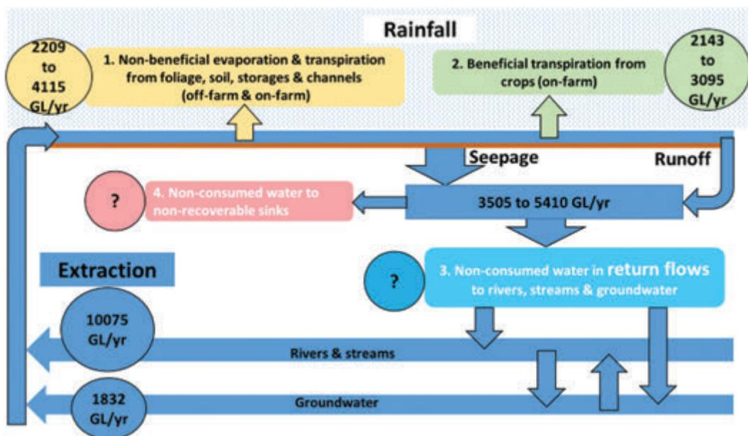
Figure 3. Illustration of the pathways of water flows and the water consumed in an irrigation district using the terminology of the International Commission on Irrigation and Drainage (Perry 2011). The approximate magnitude of these flows in the Murray-Darling Basin are derived from data in Williams (2003), CSIRO (2008), Rendell et al. (2020) and CSIRO and NSW Government (2005).
