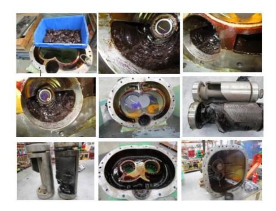
Drive Coupling Replacement by a non-qualified repairer
