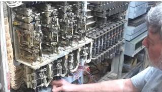
The above left is a picture<sup>28</sup> of part of a bank of bi-motional switches. Note the three banks of contacts in the lower portion of the picture and the extensive mechanical / magnet structure in the upper portion to manipulate the switch contacts.
