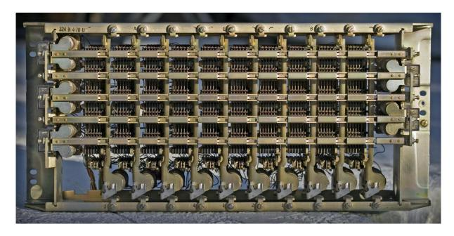
In comparison to Step-by-Step, Crossbar telephone switching technology was very low maintenance and very compact.
