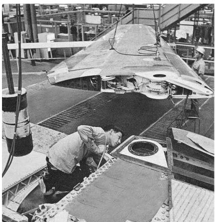
This image above gives an indication of the thickness of the wing from a side perspective to give an idea of the limitations on seeing and gaining access of the internal space. Unfortunately, I never took any photos of the work. It wasn't necessary and we signed off on the work under the Deseal/Reseal
