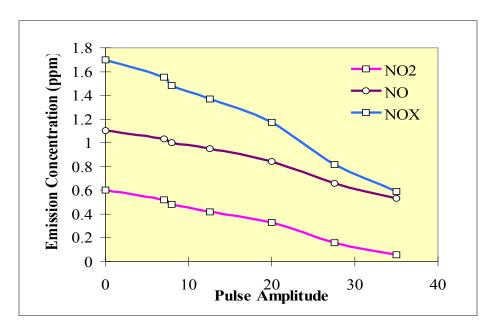
The above figure shows what happens to the NOx in a flame as the amplitude of the pulsing is increased. This causes two things to happen:
