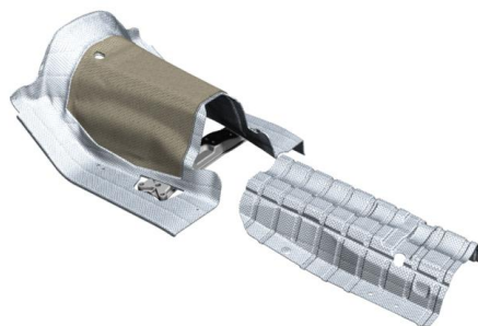
Typical Transmission Tunnel Insulator and Intermediate Heat Shield
