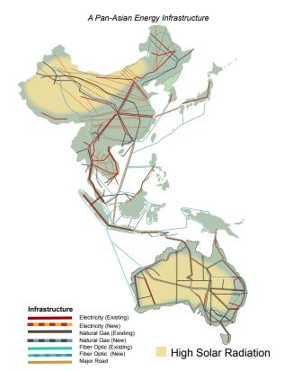
A Pan-Asian Energy Infrastructure could stretch from Australia to China. It would combine High-Voltage Direct Current power lines, natural gas pipelines and fiber optic cables.
