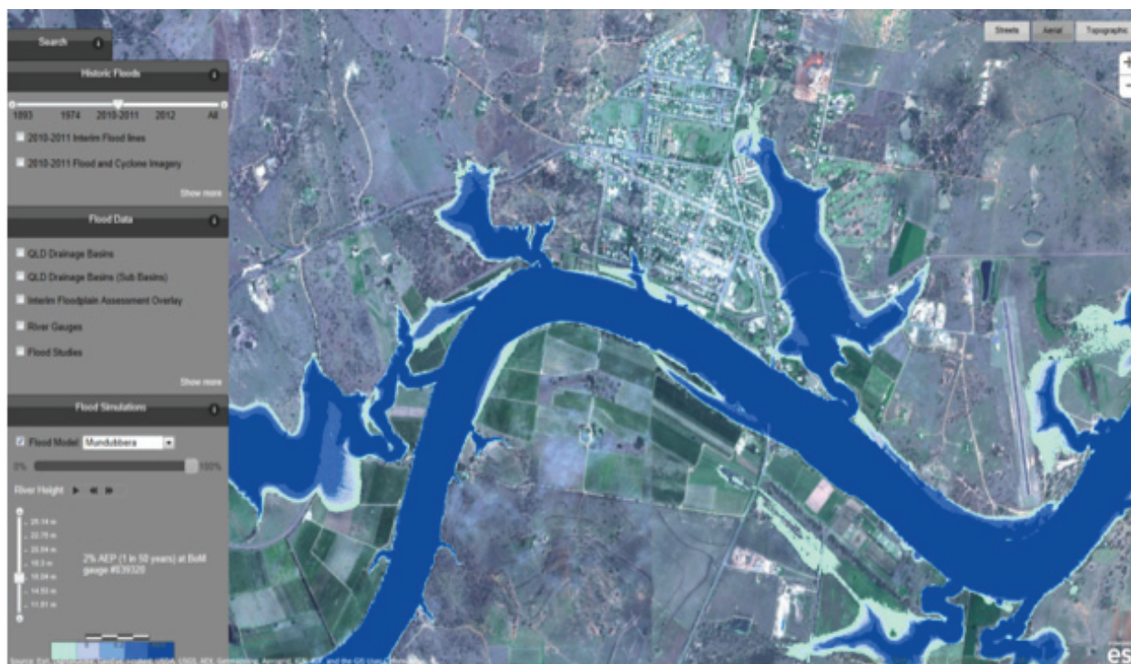
Figure 9: Mapping publicly available on the FloodCheck website shows imagery and floodline of historic events, state-wide floodplain mapping, downloadable flood information reports, and level 2 flood mapping, reports and simulations for 104 towns.
