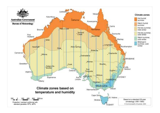
Figure 1. Blue lined areas (added by author) have potential for evaporative cooling. Region around NSW central coast and Sydney is marginal, but indirect evaporative coolers permit operation in some marginal regions.
