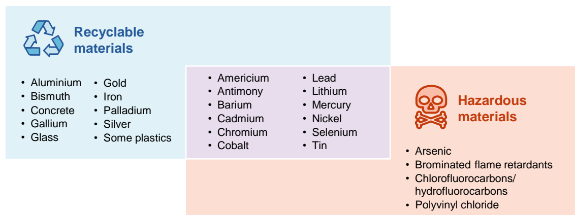
Figure 7.5 Examples of recyclable and hazardous materials in e-waste
